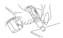
You can use cutting discs fitted to battery-operated screwdrivers or angle grinders, electrical drills as an alternative.
